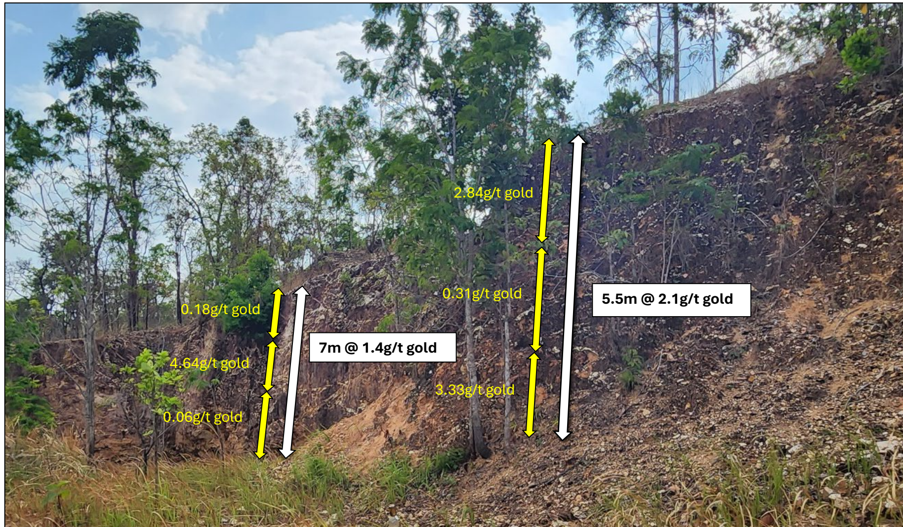
Unity channel sampling of stockwork vein mineralisation hosted in granodiorite at Camp Prospect
