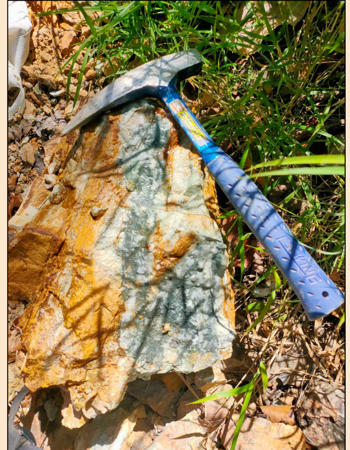
Sheeted quartz (~50%) & arsenopyrite (~50%) vein hosted in sediments. The sample is not intended to be analysed therefore the Company does not have assays. Visual estimates of mineral abundance should never be considered a proxy or substitute for laboratory analyses where concentrations or grades are the factor of principal economic interest. Visual estimates also potentially provide no information regarding impurities or deleterious physical properties relevant to valuations.
