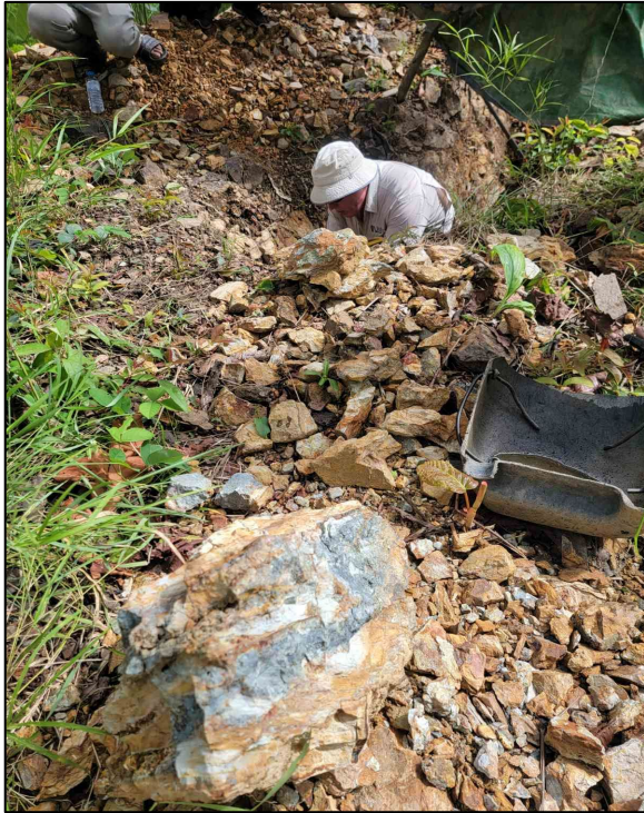
Recent artisanal workings on a 40cm wide, sheeted quartz-arsenopyrite vein hosted in sediments. A grab rock chip sample (ID 103031) taken from this vein at location Easting 694975 m, Northing 1392696 m returned 5.9 g/t gold (refer to Unity Prospectus for all rock chip assay results).
