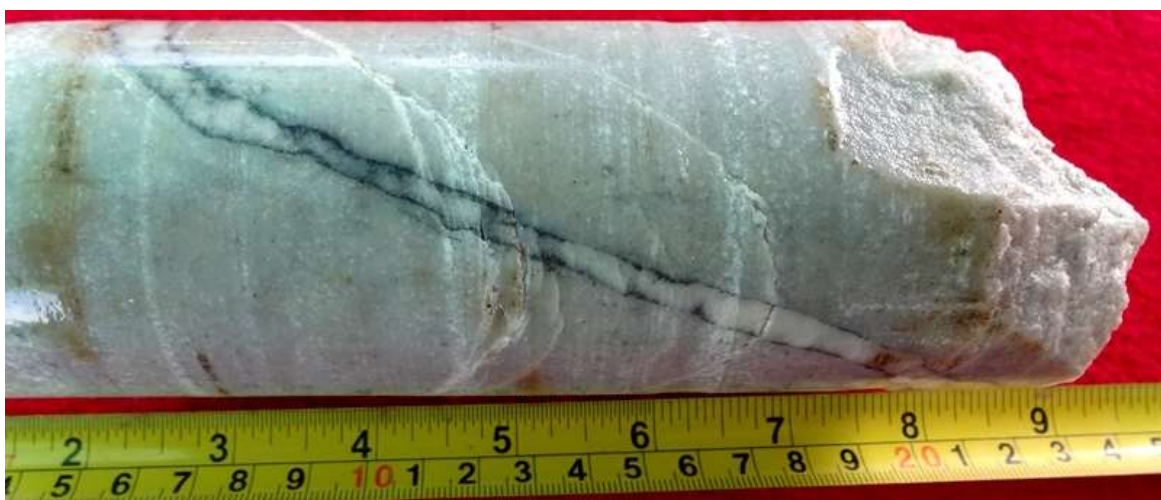
Figure 2 – (Drill Depth 283.35m) Quartz-pyrite-chalcopyrite-sericite veinlet. 6mm wide in strongly pyritic altered andesite tuff with disseminated pyrite.
