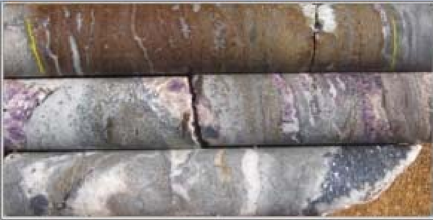
Core from Hole DF2 shows massive sphalerite, fluorite and galena
