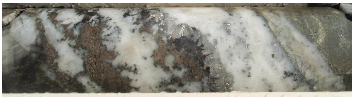
Plate 1: Sphalerite (brown), arsenopyrite (silver) and pyrite (gold colour) in a 50cm wide quartz vein (white) at 411m in CUTBD02. Field of view 16cm.
