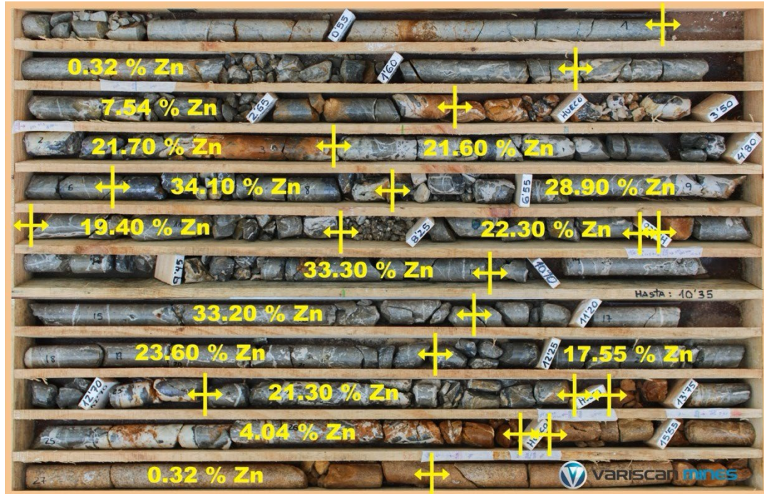
Figure 4. Diamond Drill Core from NDDT059 (15.3m @ 17.42% Zn, 4.40%) illustrating massive sphalerite hosted in dolostone. Hole depth shown is from 0.00m to 16.95m
