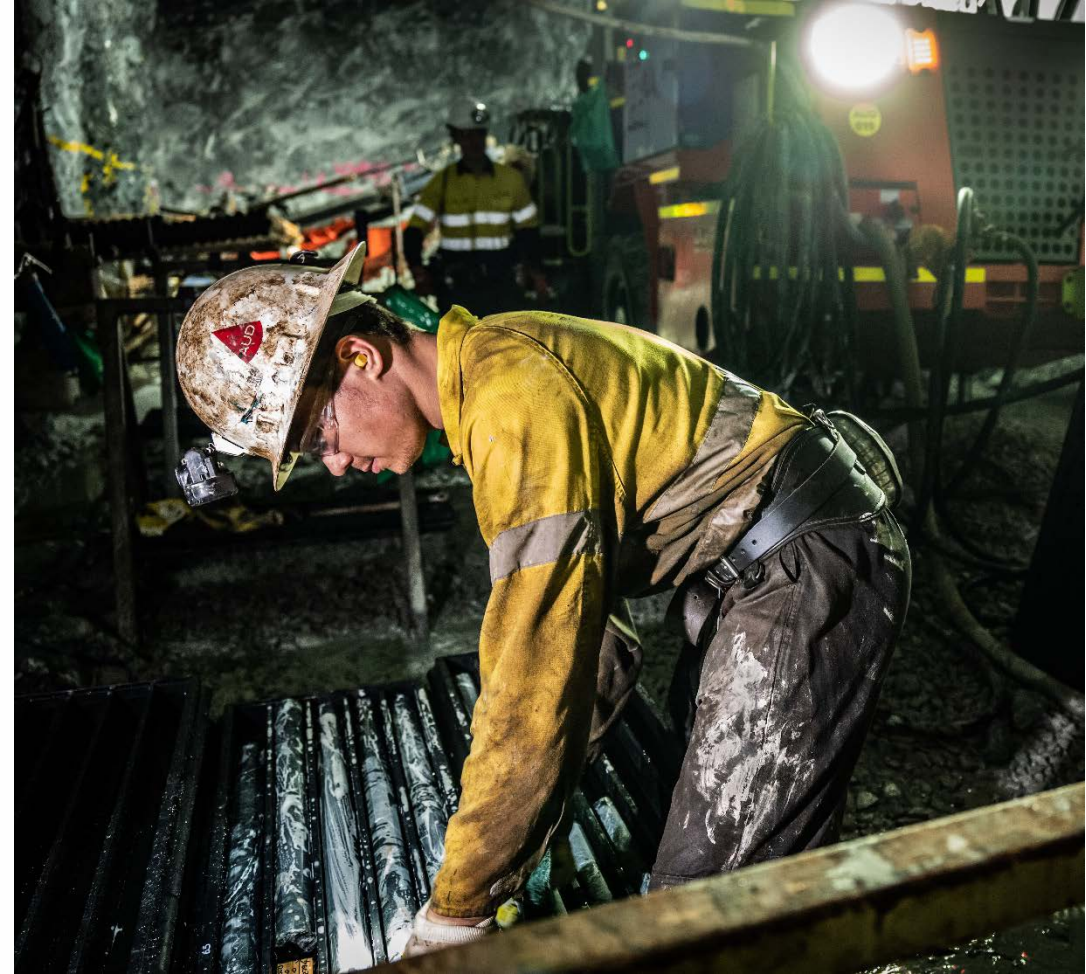
KOTH underground diamond drilling Driller's offside cleaning core after retrieving from core tube, before placing in tray
