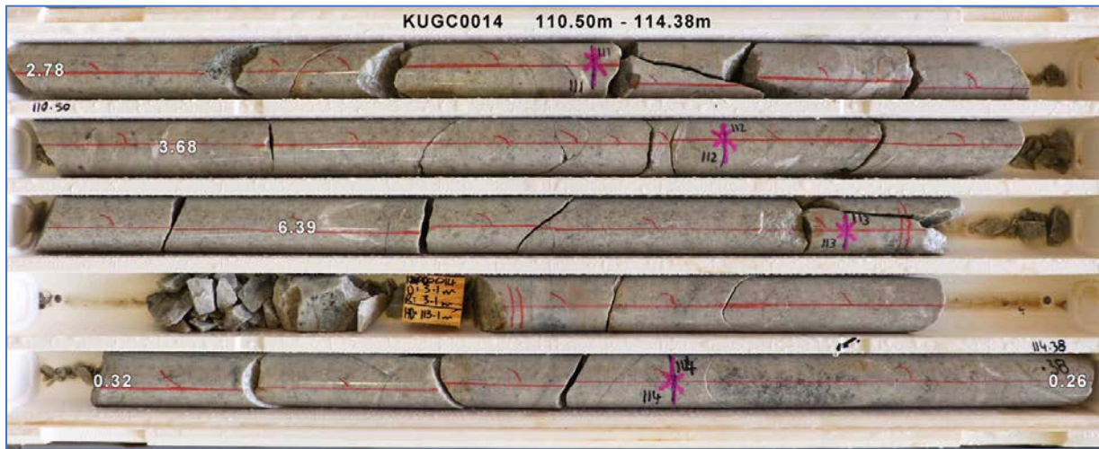
KOTH underground diamond drillhole KUGC0014 displaying typical bulk ore zone comprising quartz veinlet stockwork and gold grades (g/t)
