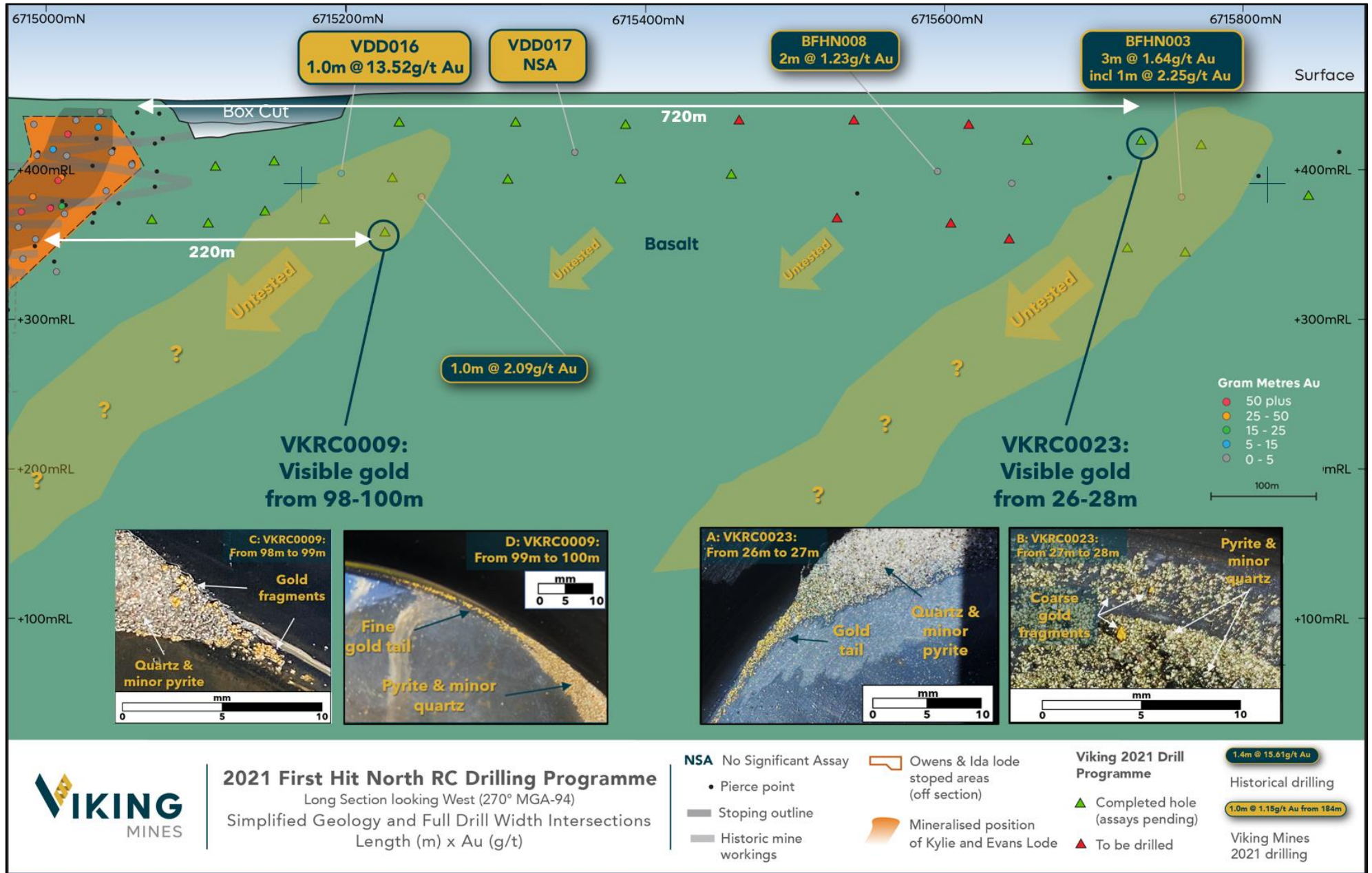
Figure 4: Long section showing location and status of RC drilling programme with completed drillholes shown and location of visible gold observed in RC drill chips. No assays have been received to date for this RC drill programme
