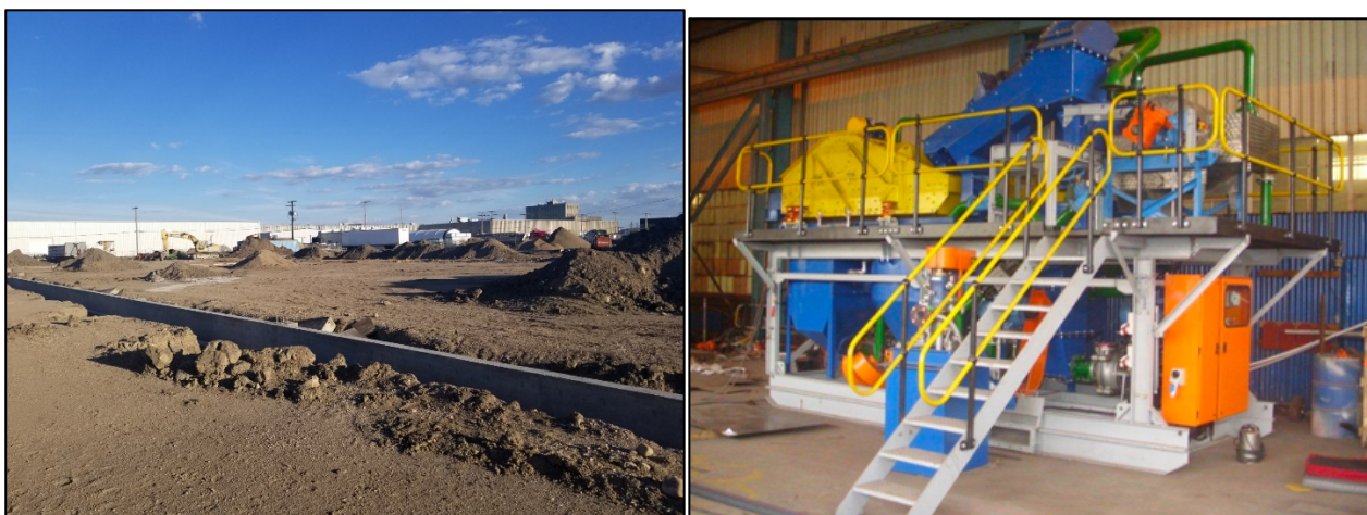
Figures 2 & 3 - Construction is underway on Vital's rare earth extraction facility in Saskatoon, which will incorporate a Dense Media Separator (right) in the extraction process
