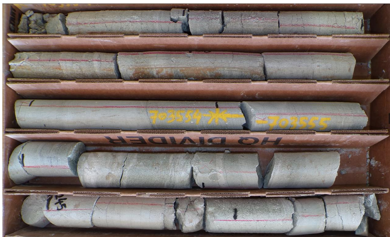
Figure 2. High-grade clay rich RMDD003 drill-core sample 703544 72.2-73.8m (237-242ft) assayed 5,150ppm Li.
