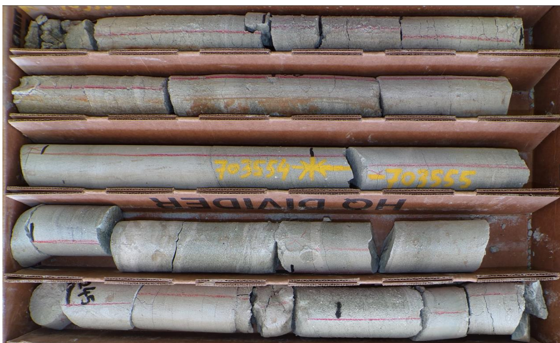
Figure 3. High-grade clay rich RMDD003 drill-core sample 703544 72.2–73.8m (237–242ft) assayed 5,150ppm Li.
