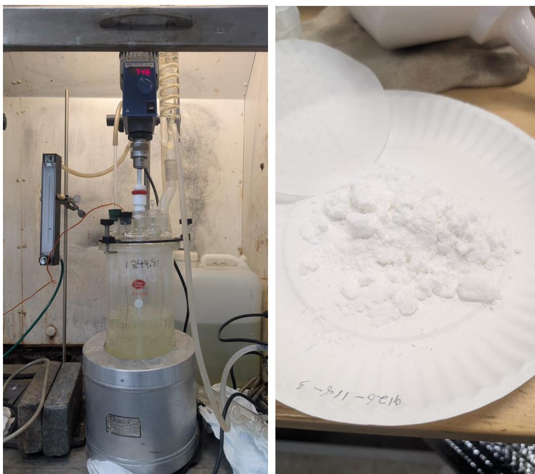
Figure 2. Precipitation apparatus (left) and first-stage precipitated lithium carbonate (right)
