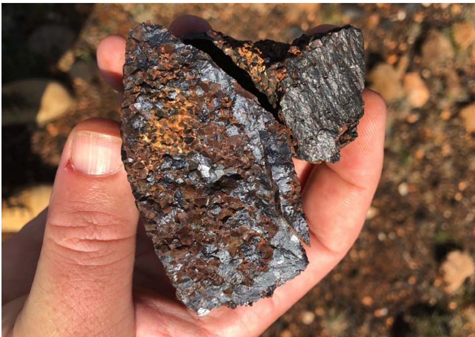
Figure 3. Hand specimen of vanadiferous titanomagnetite from the SPD Vanadium Project.
