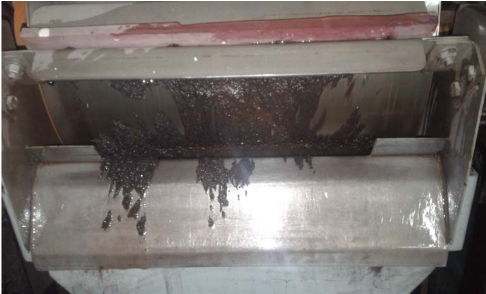
Figure 1. Magnetic concentrate from the SPD Vanadium Project.
