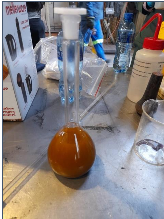
Photo 3 – Leach liquor containing dissolved Vanadium
