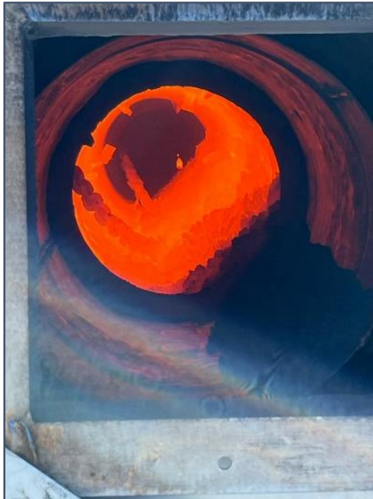
Photo 2 – Salt Roasting of concentrate
