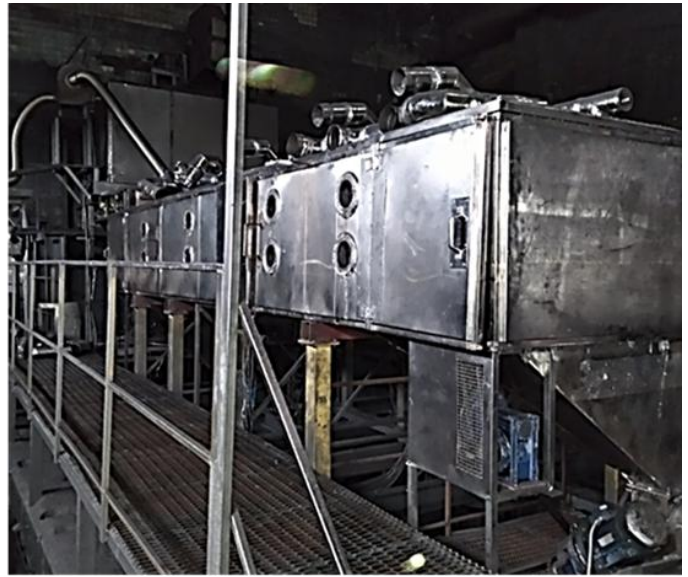
Figure 1: Zavalievsky Graphite purification circuit used to produce 99.5% HPG in Ukraine.
