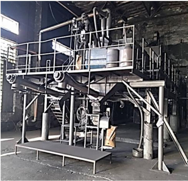
Figure 1: Zavalievsky Graphite purification circuit used to produce 99.5% HPG in Ukraine.
