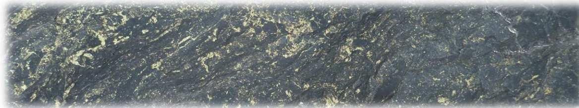
THDD236 – disseminated chalcopryite in a graphitic shale, 405m down hole, interval assayed 6.22% Cu over 1m.
