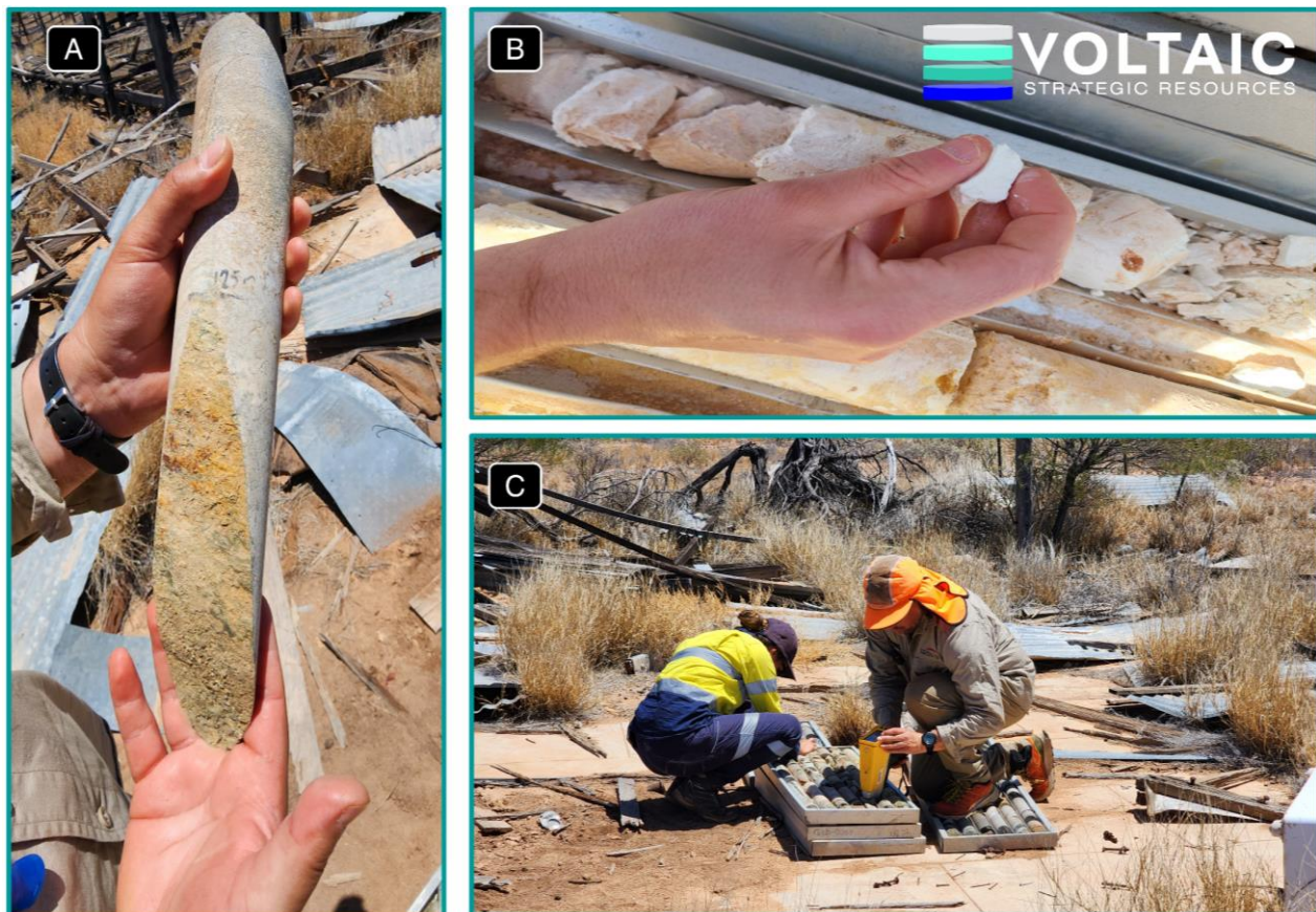
Figure 5: (a) Section of historical drillcore with elevated REEs within primary basement rock, (b) Section of historical core with elevated REEs in kaolinite clay horizon, (c) Voltaic's team confirming REE anomalism utilising pXRF
