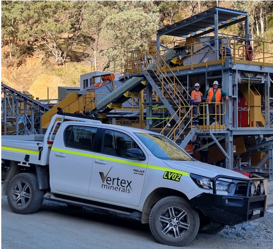
Figure 4 Ore sorting circuit
