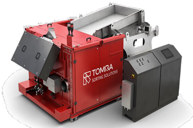
Figure 6 Picture of the Tomra laser sorter
