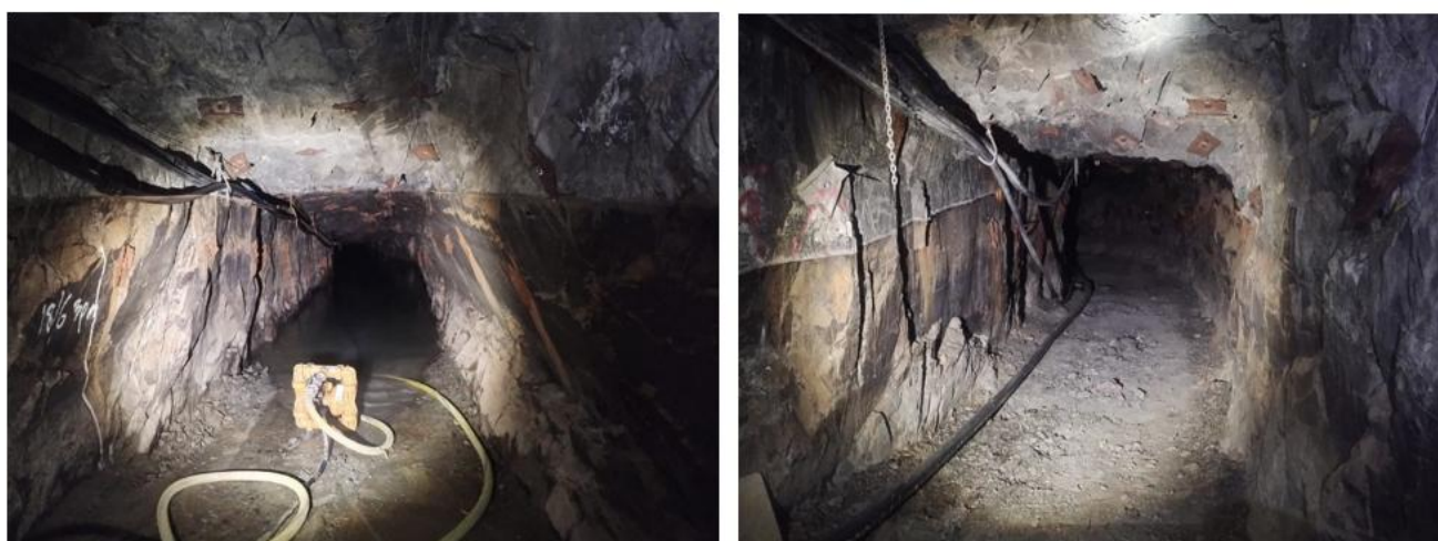
Figure 5 Mica Lense decline now dewatered. One of three gold bearing declines that carry reef gold and will be mined by flatback mining methods.
