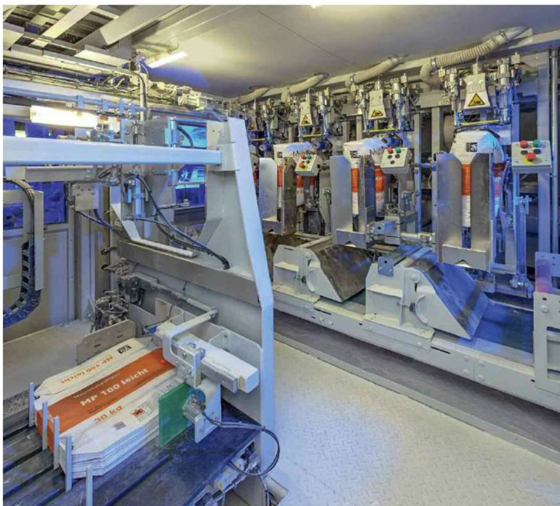
Figure 1. Haver & Boecker New HAVER M-Series 4W + B-APP 4 for Kaolin Clay
