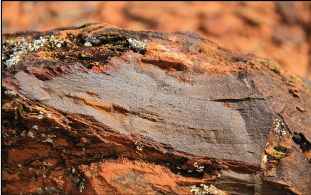
Figure 8. Typical Specimen of Hematite/Goethite Enriched DSO
