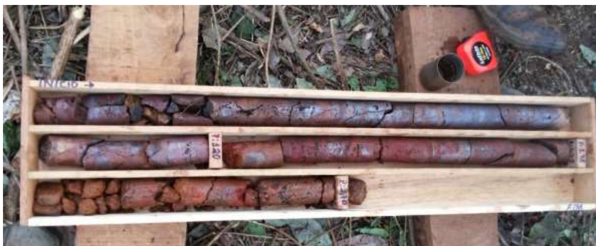
Figure 6. Massive hematite and magnetite in UJD-hole 005
