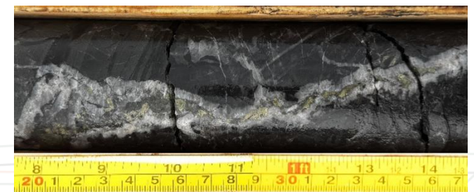
Example of chalcopyrite-bornite hosting quartz-carbonate veining within the lower Rae Group sediments of STK25001 between 181.30 and 181.52m downhole. Core diameter is NQ2.
