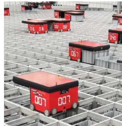
Swisslog robot carts at Catch Group warehouse
