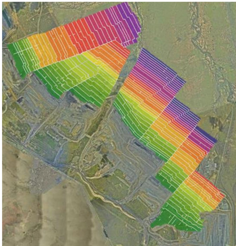
Figure 10 Example of Blackwater strip optimisation
