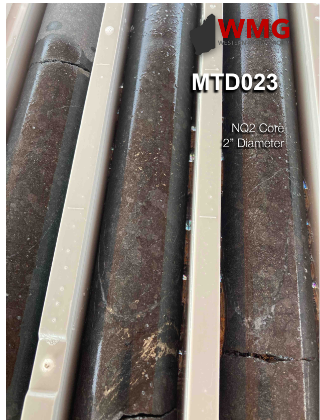
Figure 1: Photos showing examples of visible disseminated sulphides in hole MTD023 with disseminated sulphide forming interstitial blebs between olivine grains Note: core is NQ2 being 2 inches or 50mm diameter
