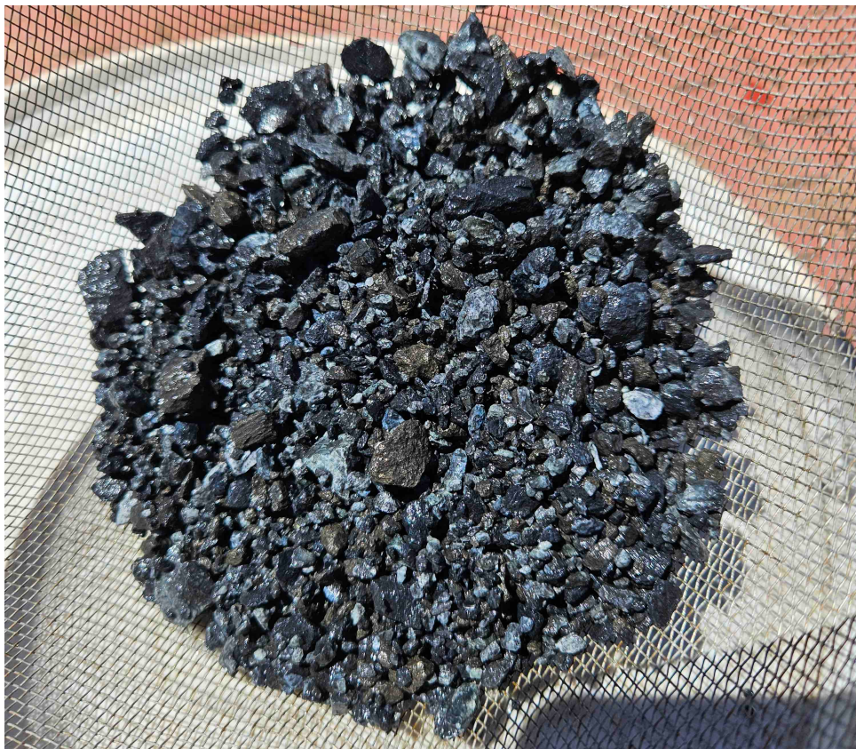
Figure 1: Example of semi-massive sulphide in RC drill chips hole MTRC024 (254-255m)
