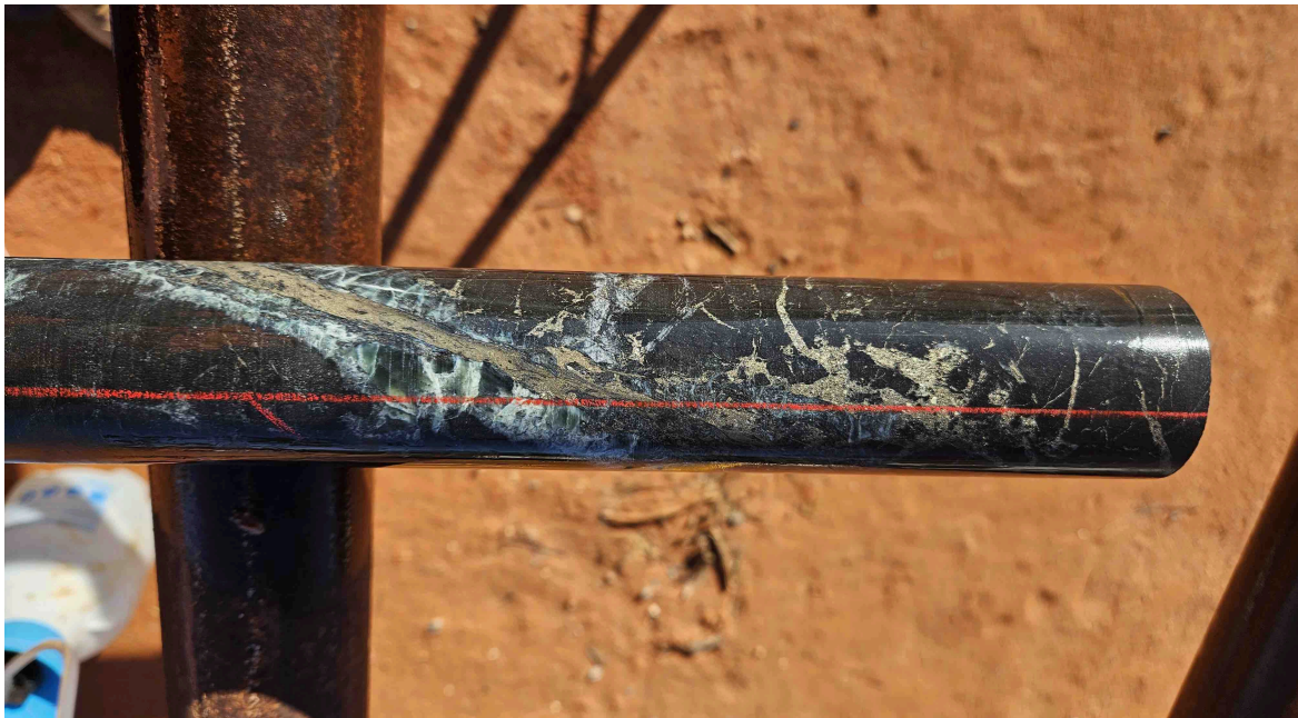
Figure 4: Example of structural vein sulphide hole MTD027
