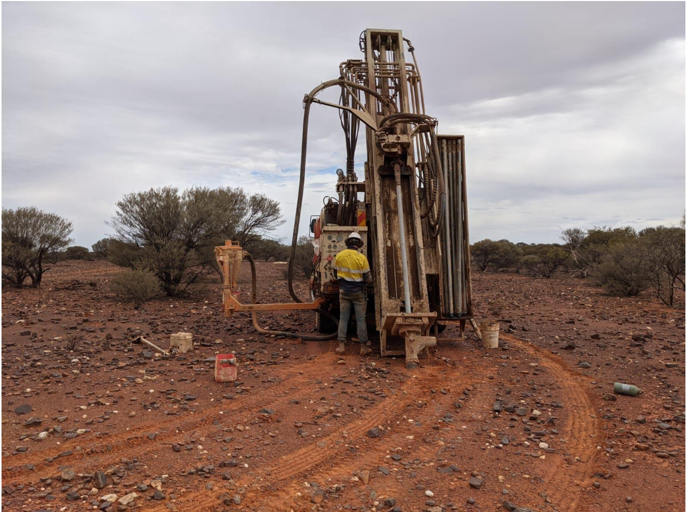
Figure 2 – Aircore drilling at the Coolallo Gold Project
