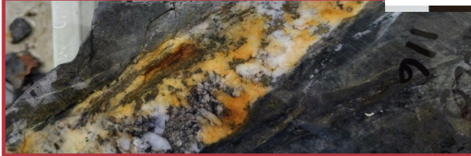
SD010 115.3m, quartz + ankerite + pyrite vein, 3.6g/t Au, 0.2% Cu (Epithermal)
