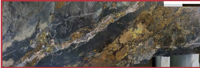
SD010 137.5m, Quartz-carbonate/ ankerite-pyrite ± chalcopryrite veins ± tellurides, sub vertical stringers, 124g/t Au, 1% Cu (Epithermal)
