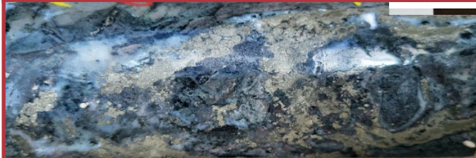
SPD003 361.8m, subvertical pyrite stringers, 22g/t Au, 0.12% Cu (Epithermal)
