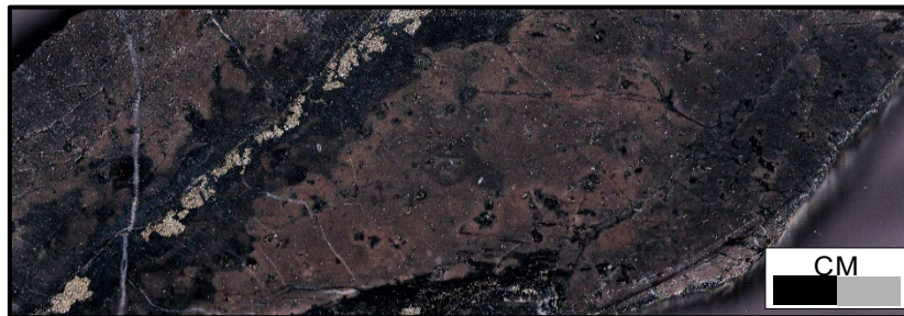
Figure 9: SPD059 – 174.2m, 1.5 g/t Au . Albitised basalt-andesite with disseminated pyrite and pyrite-carbonate veinlet with strong potassic-chlorite selvage overprinted by quartz-carbonate vein
