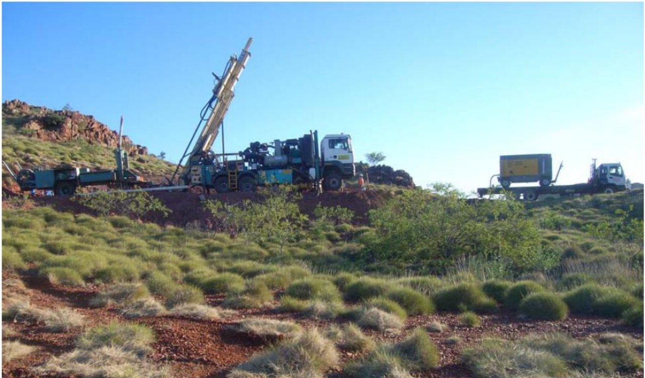
Figure 8 – RC drilling underway at Miaree Gold Project.
