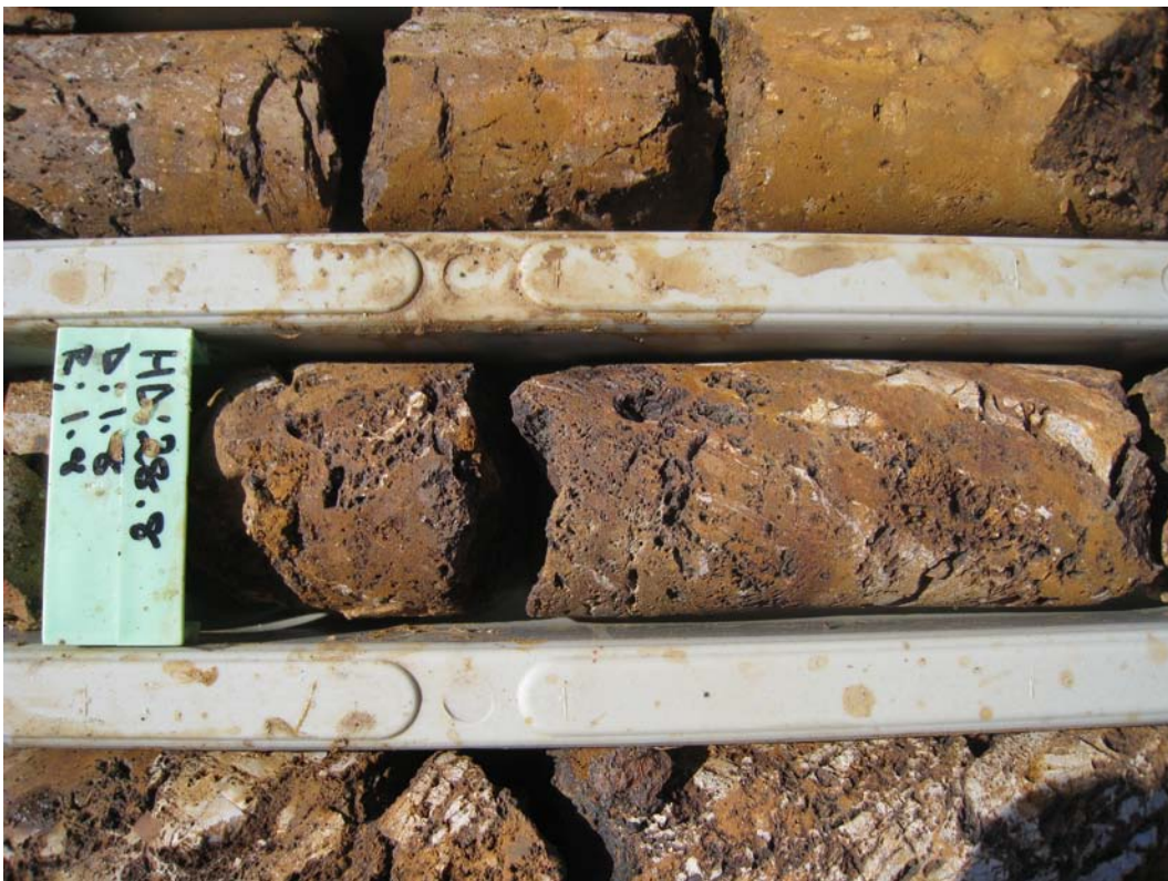
Figure 4 – Typical oxide ore from Golden Camel metallurgical hole MET3
