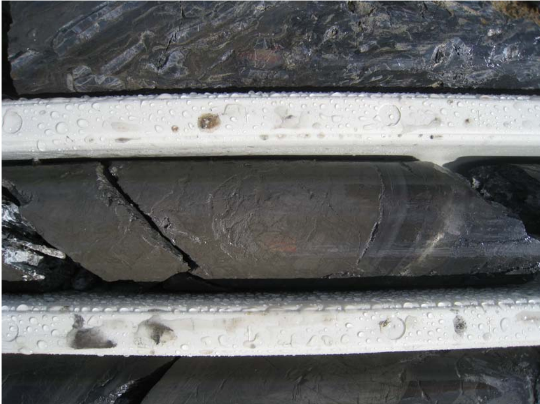
Figure 5 – Sulphide mineralisation from Golden Camel hole MET3
