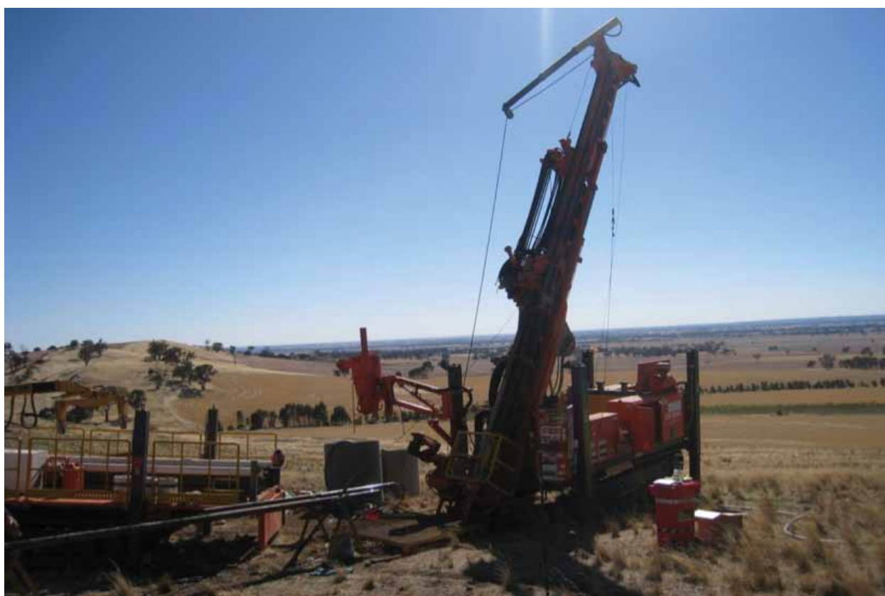
Figure 3 – Drilling geotechnical hole GTC2 at Golden Camel
