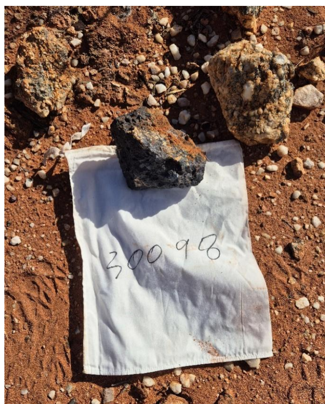
Figure 3 – Co-Ni-Cu-Pb-Sc mineralisation within hematite-quartz yielding 2.47% Co, 0.58% Cu, 1.07% Ni, 1.30% Pb, 126.25 ppm Sc 2 O from sample 30098
