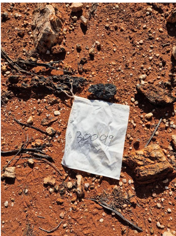
Figure 2 – Co-Ni-Cu-Pb-Sc mineralisation within hematite-quartz yielding 0.95% Co, 0.29% Cu, 0.42% Ni, 0.41% Pb, 97.8ppm Sc 2 O from sample 30099
