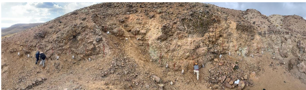
Figure 8: Channel sampling at Cobremani – 35.6m channel sample @ 1.3% Cu and 22.85g/t Ag
