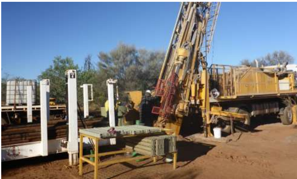
Figure 2. Diamond Drilling at EM Target #1, Mount Hardy
