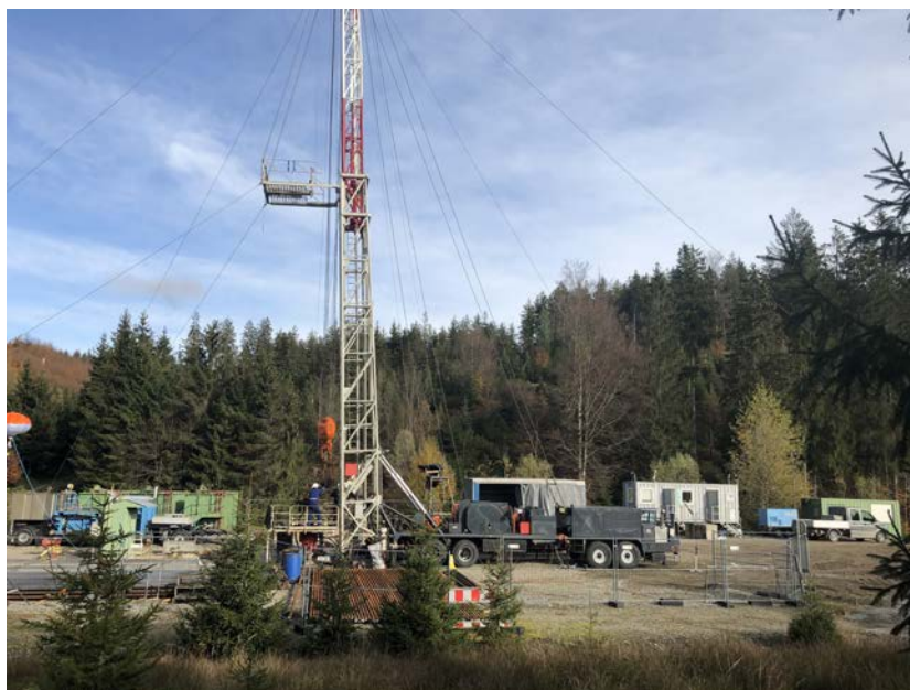
The RED W-101 workover rig undertaking operations in Upper Austria
