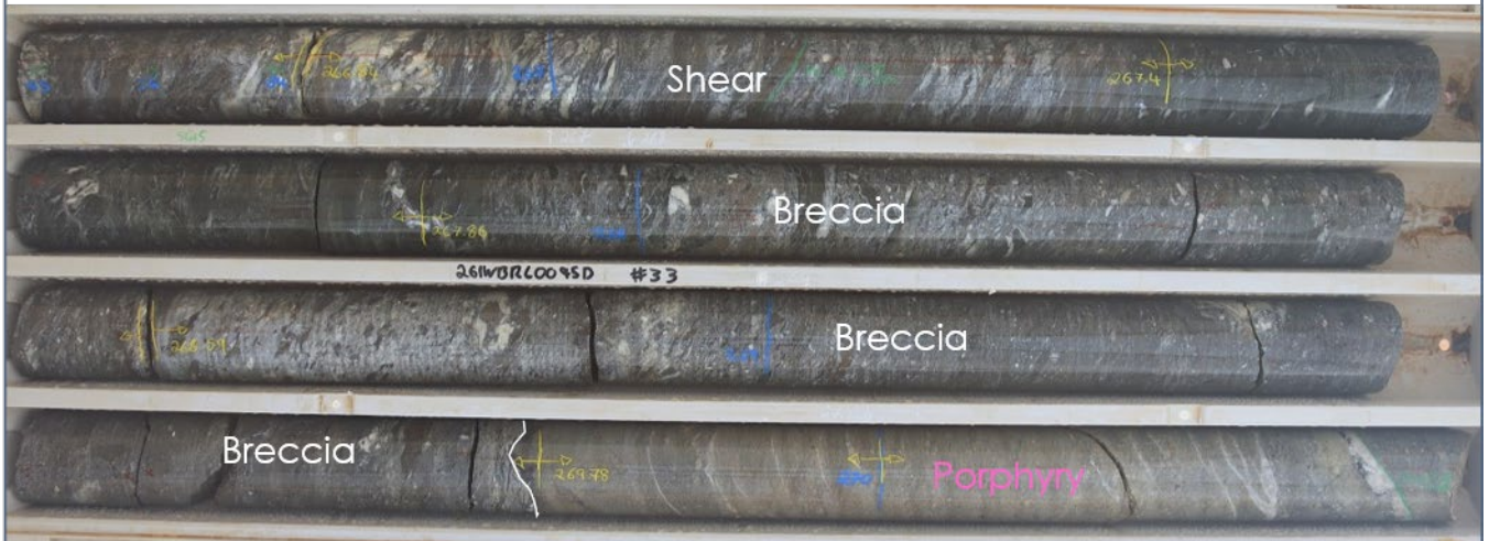
Figure 6: HQ core from 26IWBRC0095D showing an example of a heavily altered and sulphide rich brecciated sediments adjacent to a porphyry dyke observed within one of the target structures (see Table 6).
