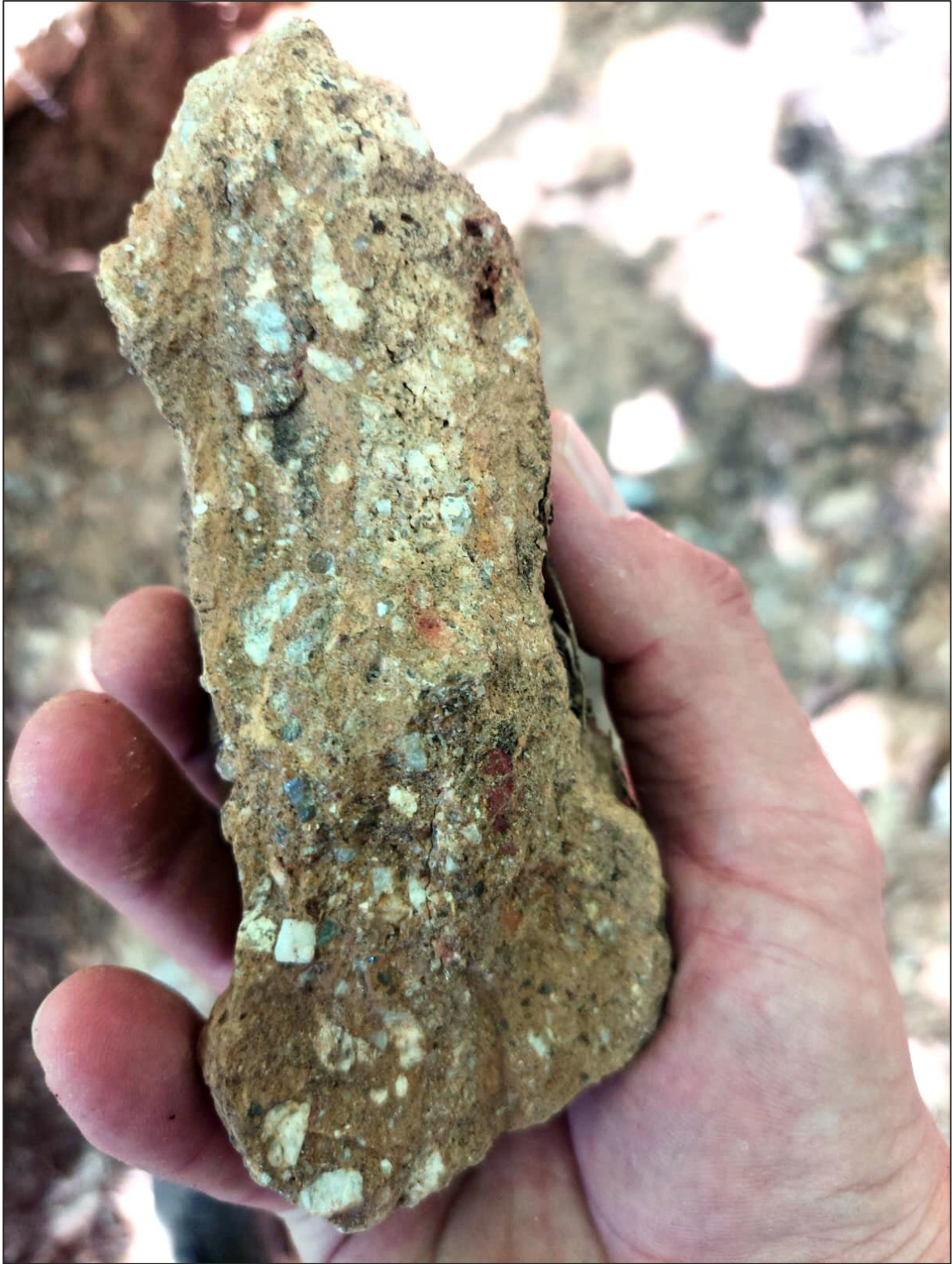
Figure 4: Zekil locality – diatreme polymict breccia, showing wispy undulating quartz-carbonate veins and feldspar/quartz comb crystal growth and gold mineralisation
