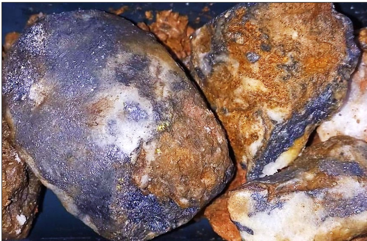
Figure 5: Drillhole KVDD001, drill core pieces (~10x5cm) showing blue-grey galena and sphalerite, with minor yellow chalcopyrite specs (interval 28.7-28.9m depth).
