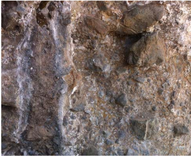
Figure 7a; Volcanic breccia of andesitic composition at the base of volcanic flows. Strong clay sulphide alteration in some areas.
