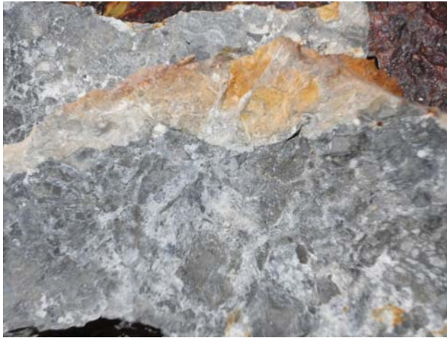
Figure 7e; Quartz-chlorite-pyrite altered andesitic rock with hydrothermal brecciation evident
