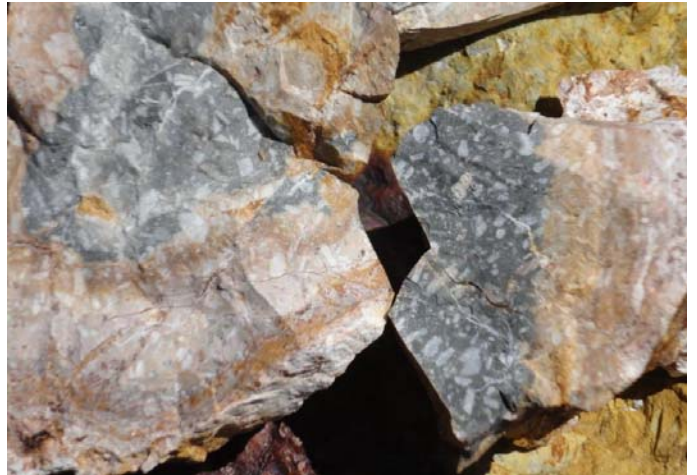
Figure 7f; Strong quartz-pyrite alteration of a porphyritic andesite
