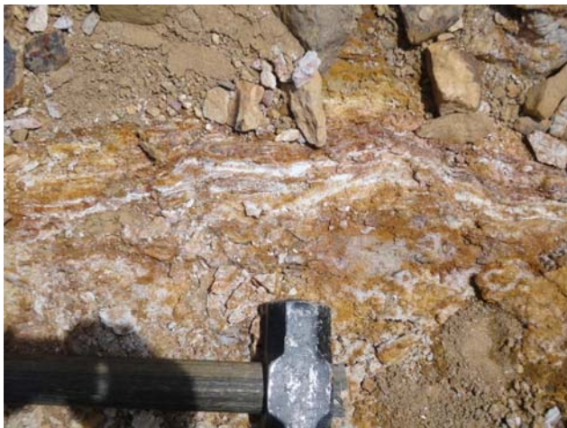
Figure 7g; Clay veins cutting argillically altered pyroclastic rocks. The veins are possibly after feldspar and altered by further-ongoing acid (argillic) alteration.
