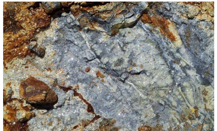
Figure 7d; Disseminated sulphides in strongly clay altered volcanic tuffs with possible sericite. Grey disseminated sulphides in altered rock and hematite after pyrite veins. Analysis is required to confirm clay mineral speciation.
