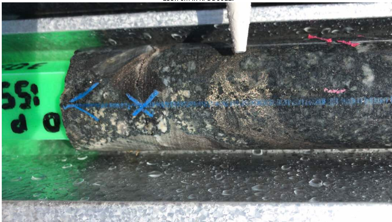
Figure 4: Semi-massive zone of pyrrhotite associated with qtz-chlorite-epidote alteration within a greenstone units from 155.70m in KPDD0012.
