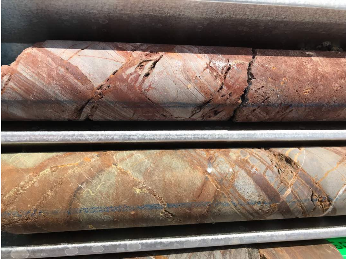
Figure 2: Zone of strongly weathered, well-developed quartz-calcite veins in a Banded Iron Formation (BIF) unit from 74.32 to 84.68m in KPDD001.
