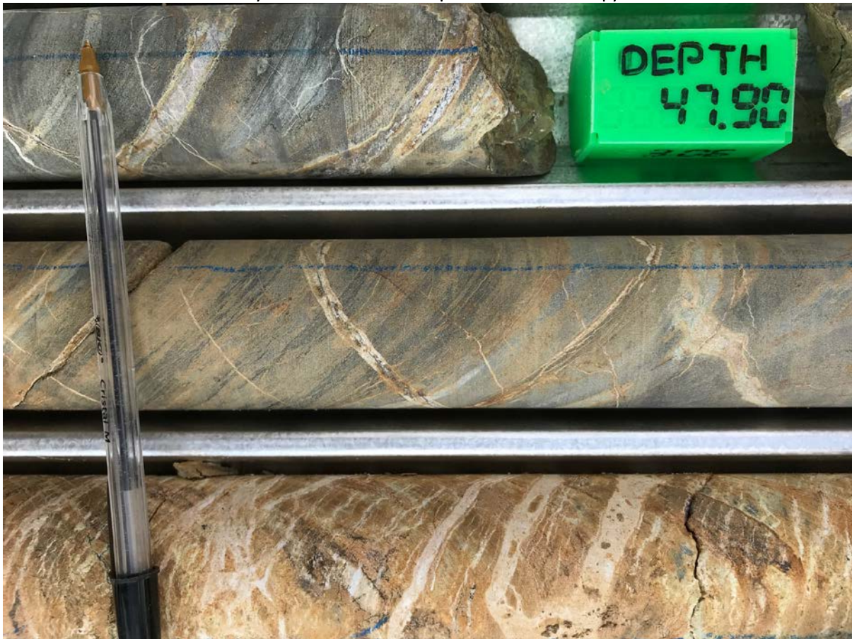
Figure 3: Close up of highly weathered zone of intense calcite-quartz veins from ~46-48m in KPDD018. Photo shows examples of rusty cubes in the veins interpreted to be oxidised pyrite.
