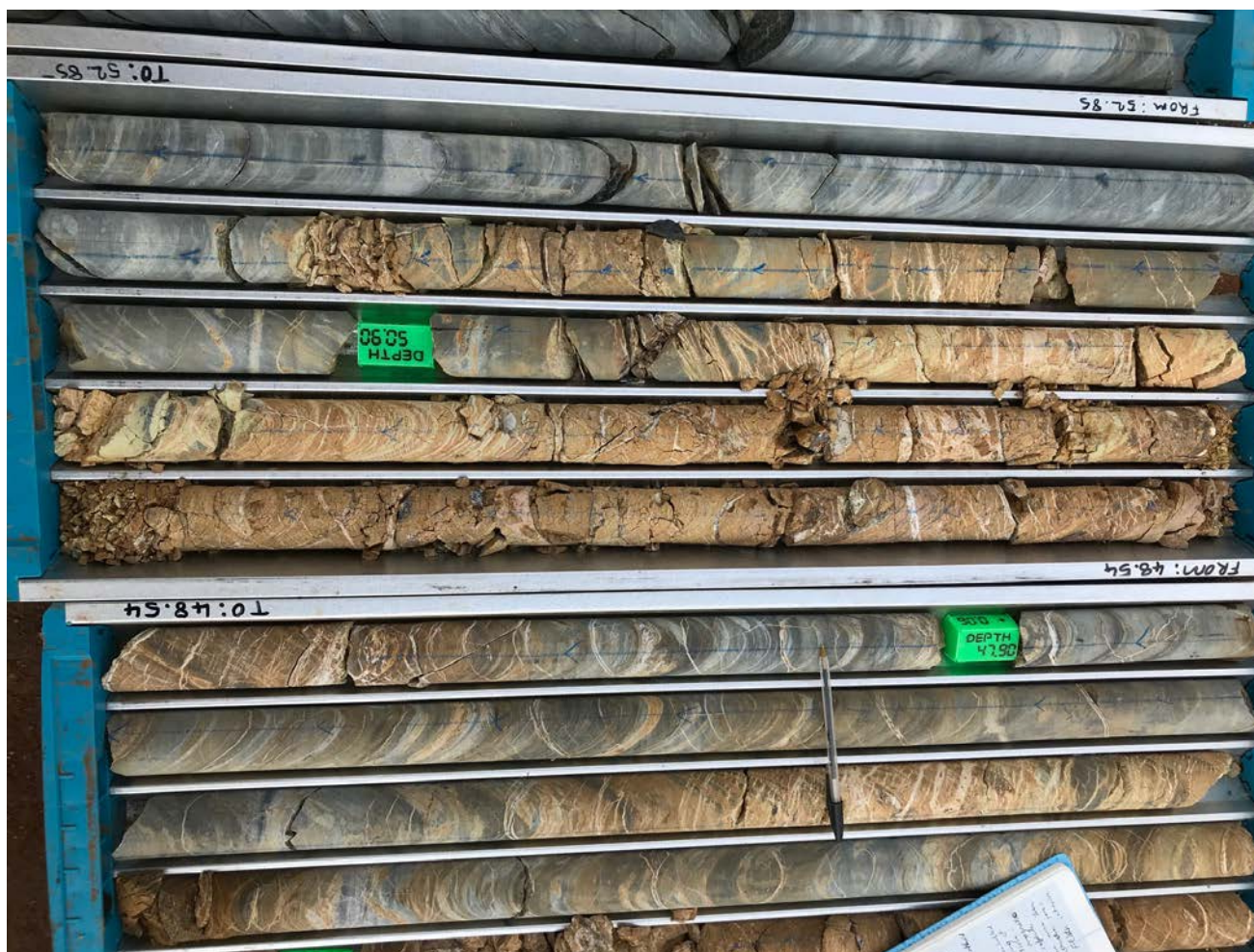
Figure 2: Highly weathered zone of intense calcite-quartz veins and associated chlorite-epidote alteration hosted within an interlayered sequence of Banded Iron Formations and greenstones from KPDD018.
