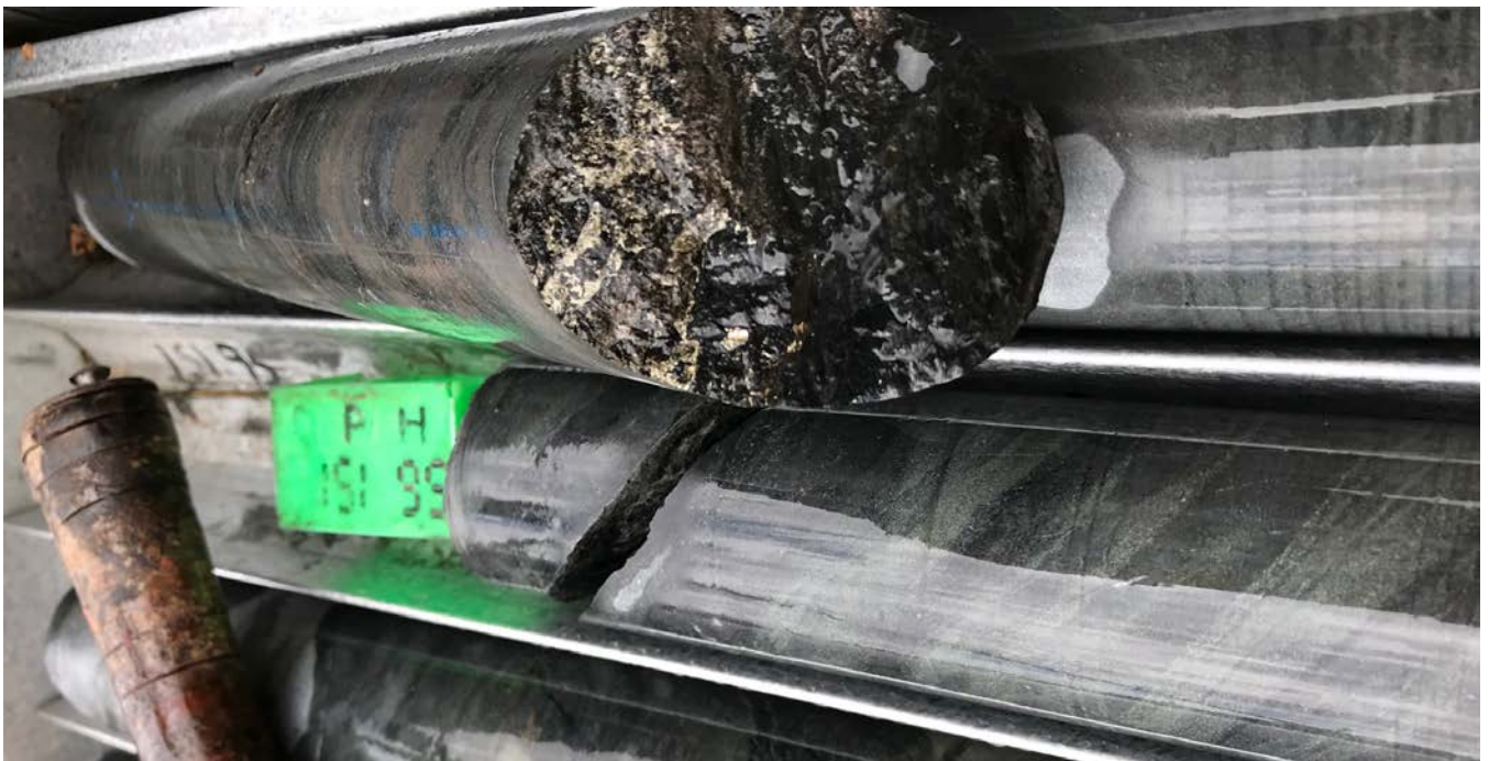
Figure 6: Disseminated to semi-massive zone of pyrrhotite associated with qtz-chlorite-epidote alteration within a greenstone/ironstone unit from KPDD0018.
