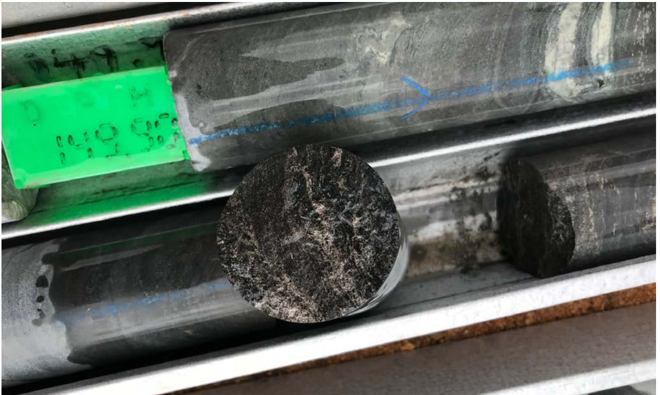
Figure 6: Disseminated to semi-massive zone of pyrrhotite associated with qtz-chlorite-epidote alteration within a greenstone/ironstone unit from KPDD0018.
