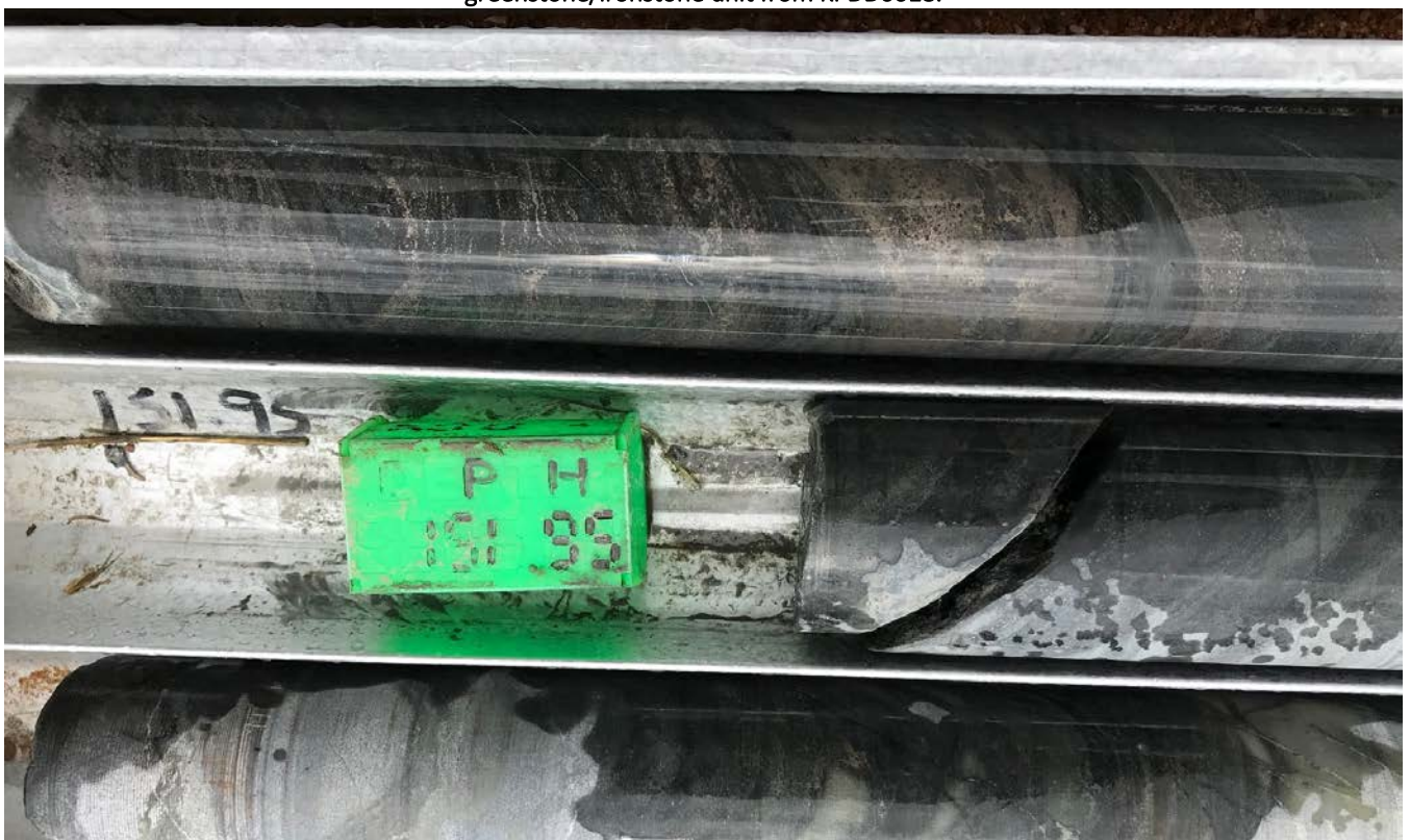
Figure 4: Disseminated to semi-massive zone of pyrrhotite associated with qtz-chlorite-epidote alteration within a greenstone/ironstone unit from KPDD0018.
