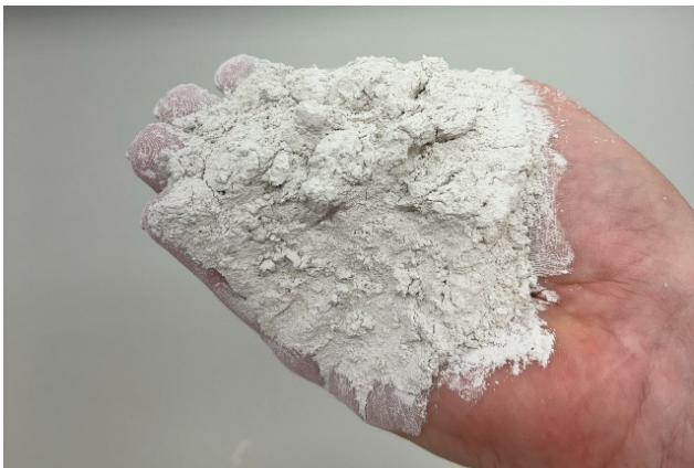
Figure 1: AusPozz™ produced from one of the pilot-scale calcination test runs
