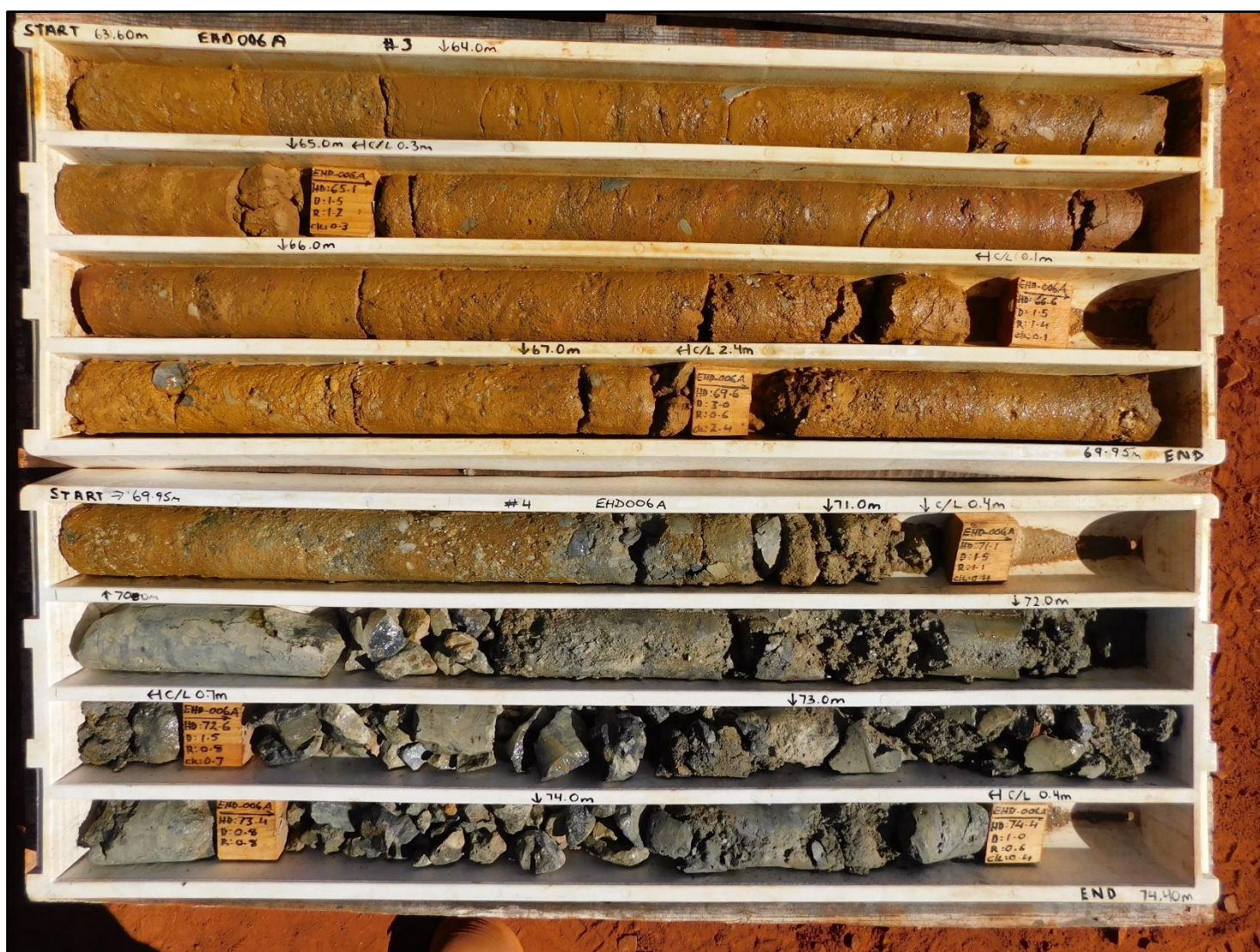
Image 5 – EHD006A – Soft sediment slumping - debris flow – (hanging wall) over partly silicified, brecciated alternating hard-soft Zn-Pb mineralisation – Facies controlled transition zone.
