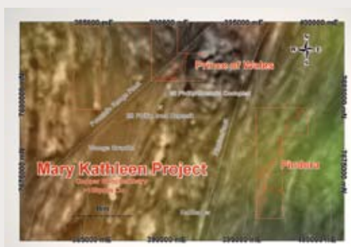
Prince of Wales and Pindora targets, areas of elevated copper geochemistry (>100ppm copper) highlighted in red. Background is regional magnetics draped over gravity.
