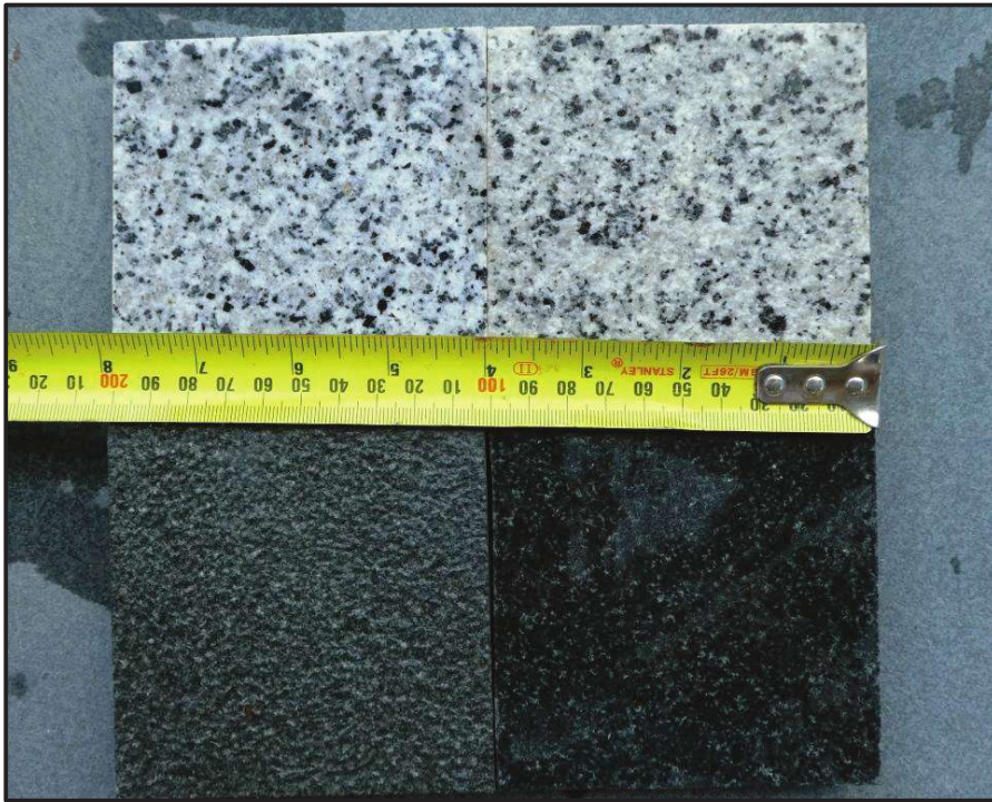
Photo 2: Prepared tiles of white granite and dark green-grey microgabbro
