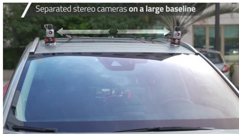
Generating 3D stereo perception from 2 separate mono cameras with different fields of view
